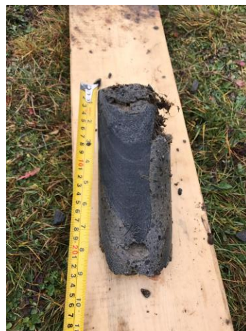
Figure 6: Extracted core samples from arch.
