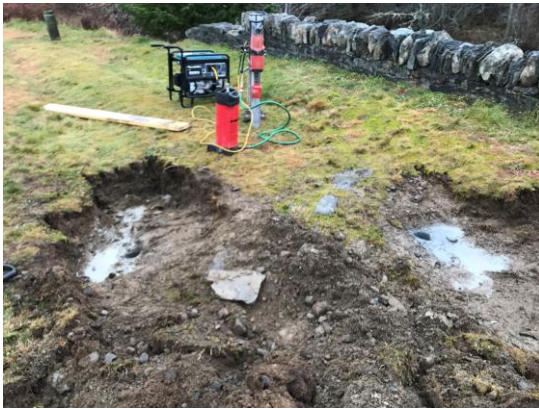
Figure 5: Masonry core extraction of arch (Left), Borehole drilling at north approach (Right)
