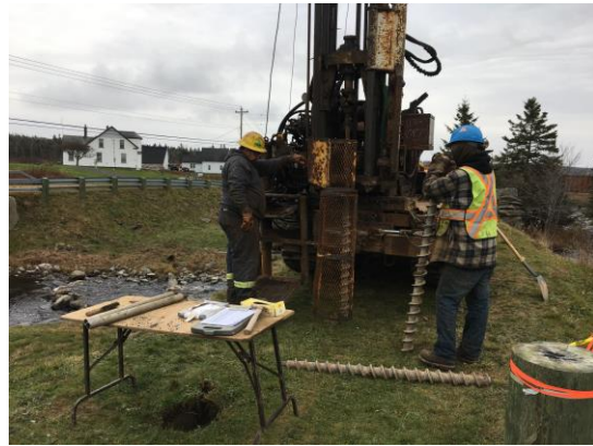
Figure 5: Masonry core extraction of arch (Left), Borehole drilling at north approach (Right)
