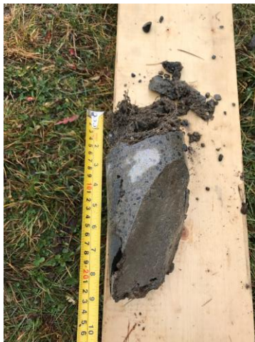
Figure 6: Extracted core samples from arch.
